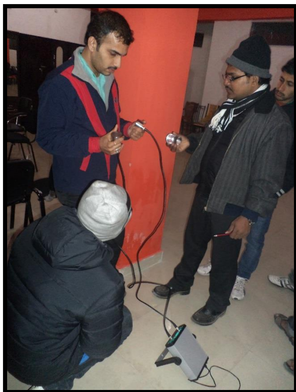
Figure 74: Ultrasonic Pulse Velocity Method (Kangra, 17th December 2013)
